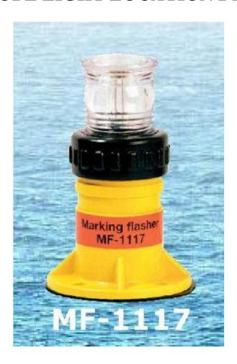
MF-1117 requires a customer own inline ON/OFF switch. High intensity xenon flash strobe light. Requires external power, 12-24V DC. Water resistant to IP 68. Flash rate: 90 flash per minute as standard. Clear lens as standard. Optional colour lenses available.
