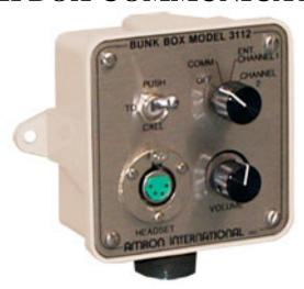
Provides communication and two entertainment channels to individual bunks. A headset is required. Communication can be push-to-talk or Simulcom. A push-to-call switch activates an indicator on an Amron Comm Routing Panel. Input connector is MS type 14 pin, male (MIL-C-5015). Headset connector is 4 pin audio, female. Housing is die cast zinc with gray epoxy powdercoat and stainless steel front panel.
